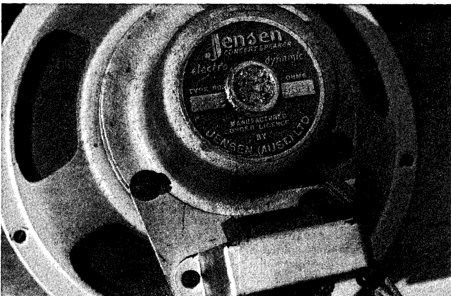
A Jensen electrodynamic loudspeaker with a 3k \Omega field coil is used in the Airking. Fortunately, both the field coil and the output transformer were in working order.
