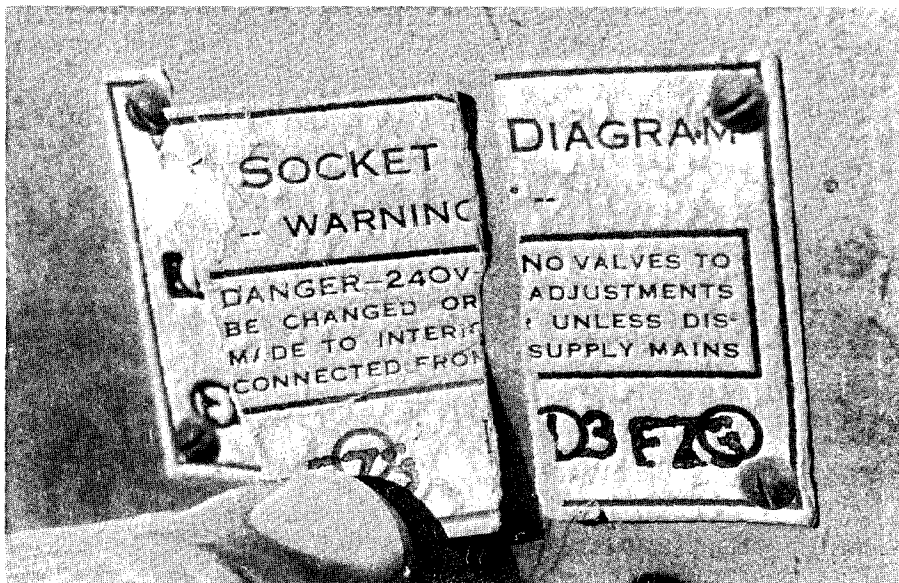
The missing section of the valve socket diagram solved the mystery of the unknown valve type. The receiver originally used an EZ3 power rectifier as a diode detector.
