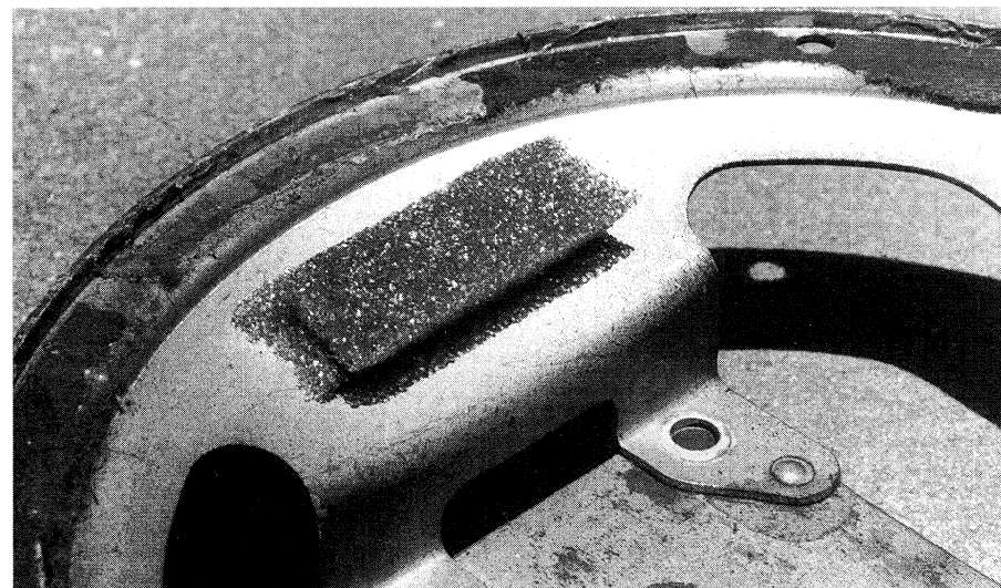
This piece (and several other pieces) of foam plastic behind the speaker cone indicate a previous attempt to eliminate the cone rattle. Because the voice coil assembly was loose, the attempt was unsuccessful.
