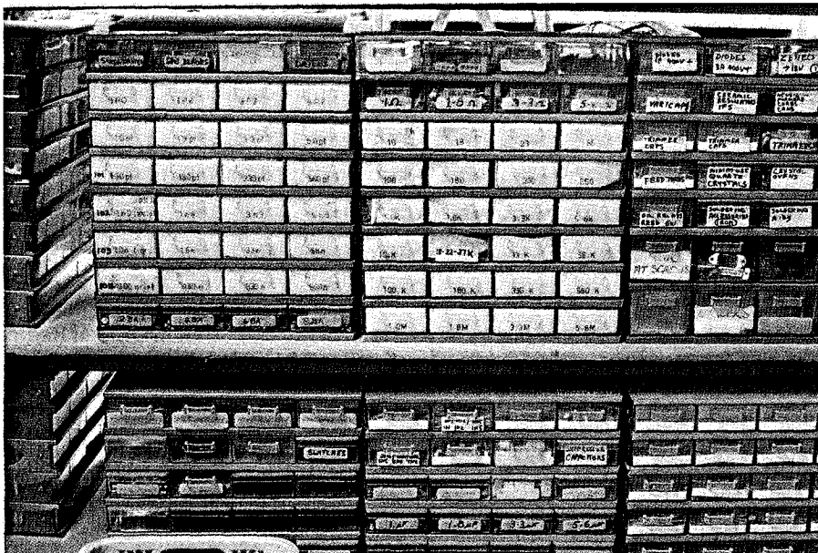
Multi-drawer parts cabinets (available from electronics retailers) are ideal for storing smaller components.
