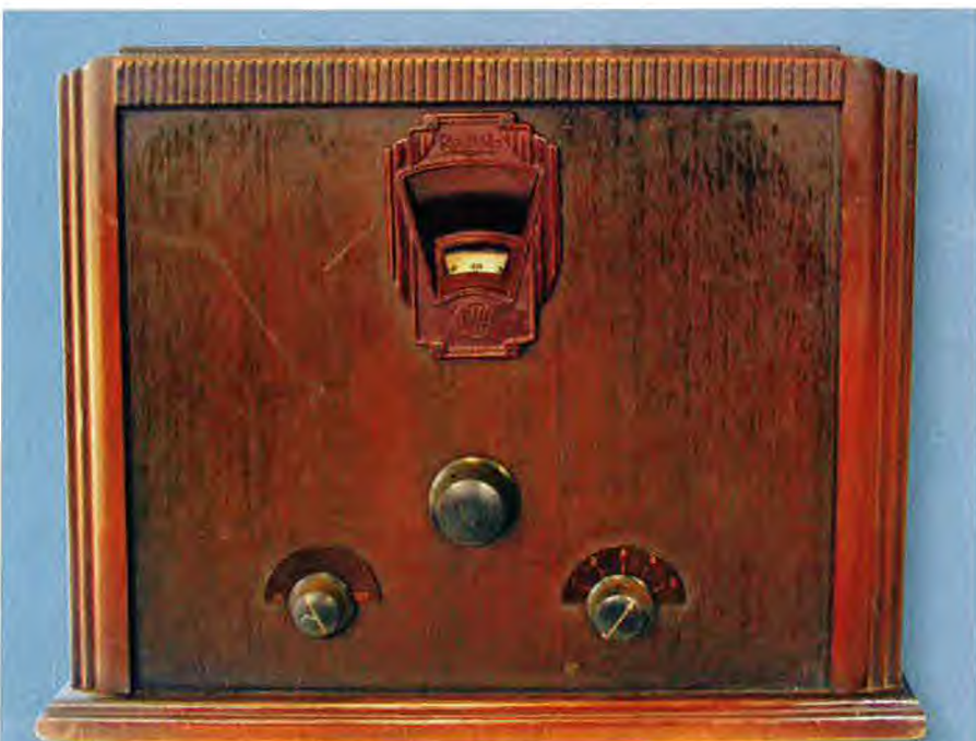
The AWA C103/43 shortwave converter is housed in a wooden cabinet. This is also in good condition and will be easy to restore.
