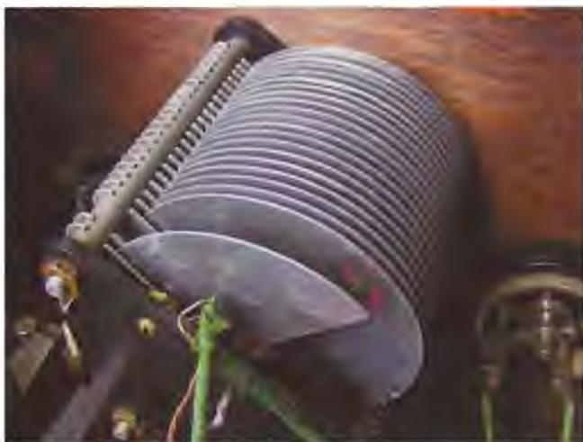
The tuning gang is unusual in that it features an additional single moveable plate at the back which is controlled by a separate shaft inside the main tuning shaft. This allows the station frequency to be precisely adjusted when tuning.
