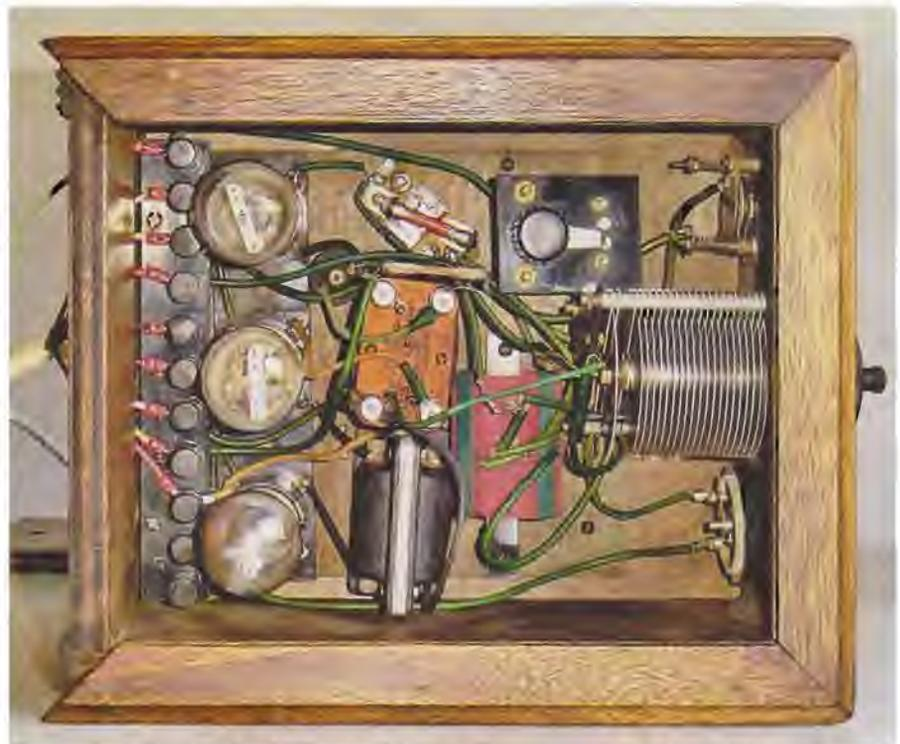
This is the view inside the set with the top cover removed. Note the breadboard style of construction, with all parts readily accessible from the top.
