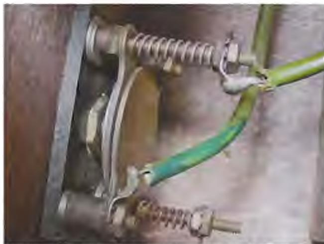
The regeneration (or reaction) control resembles a mica pad capacitor. Rotating the control knob varies the distance between the plates and thus the capacitance and the amount of regeneration.
