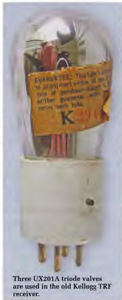
Three UX201A triode valves are used in the old Kellogg TRF receiver.
