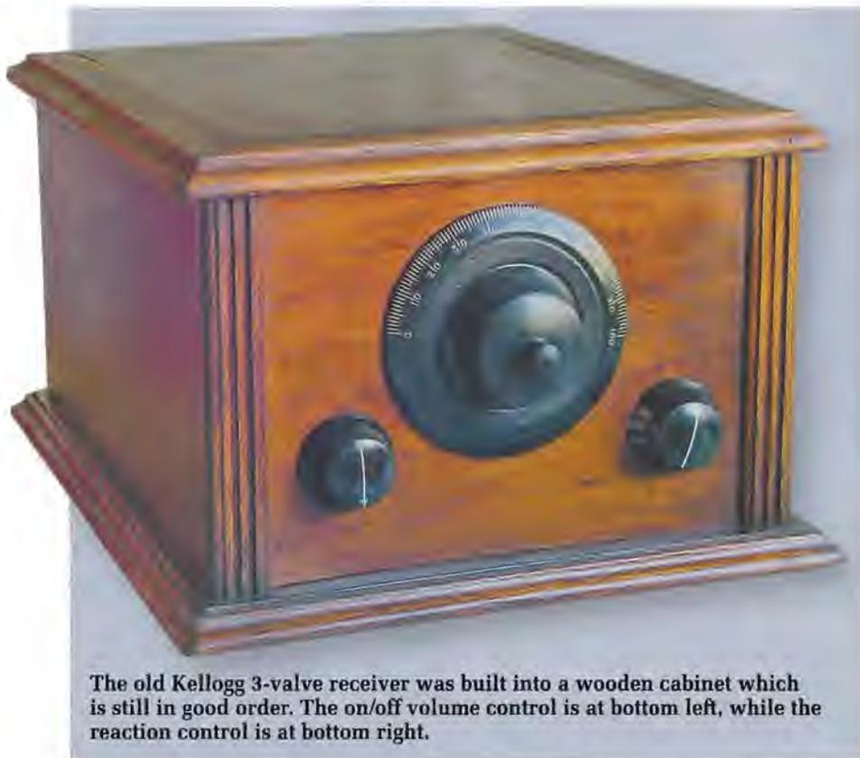
The old Kellogg 3-valve receiver was built into a wooden cabinet which is still in good order. The on/off volume control is at bottom left, while the reaction control is at bottom right.
