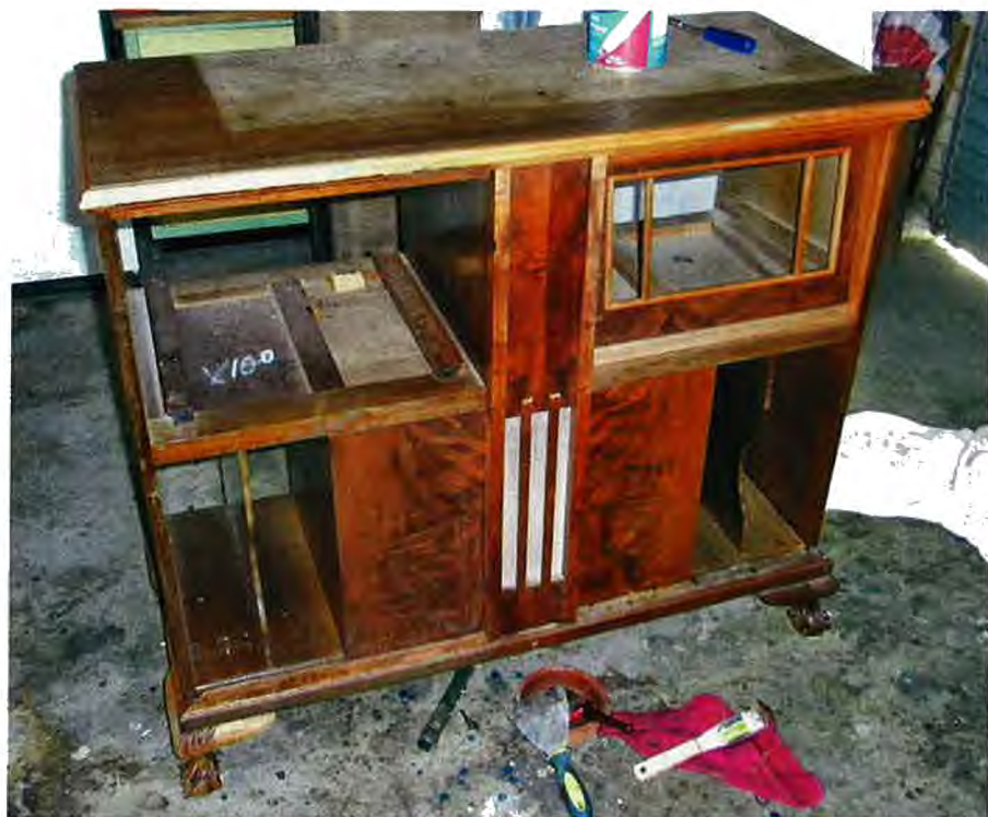
This view shows the A8551's cabinet during restoration. The timber was in good condition but the finish had deteriorated quite markedly over the years.
