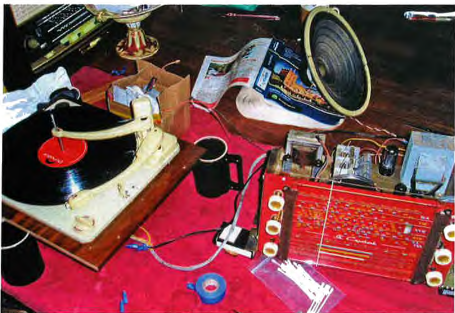
The record changer, chassis and loudspeaker were all removed from the cabinet to make the restoration easier.
