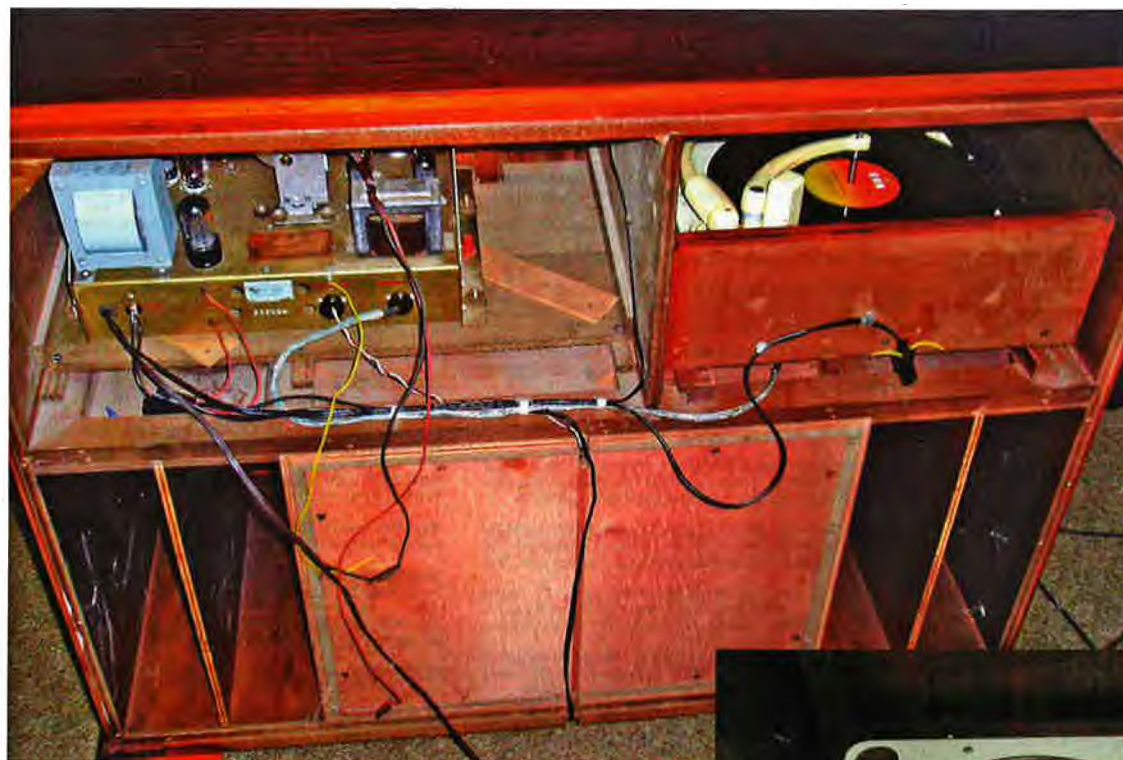
A rear view of the cabinet with the record changer and radiogram chassis mounted in position. The connecting cables between them run along a shelf at the back of the unit. This unit is much more elaborate than the average radiogram of the mid-1950s era.
