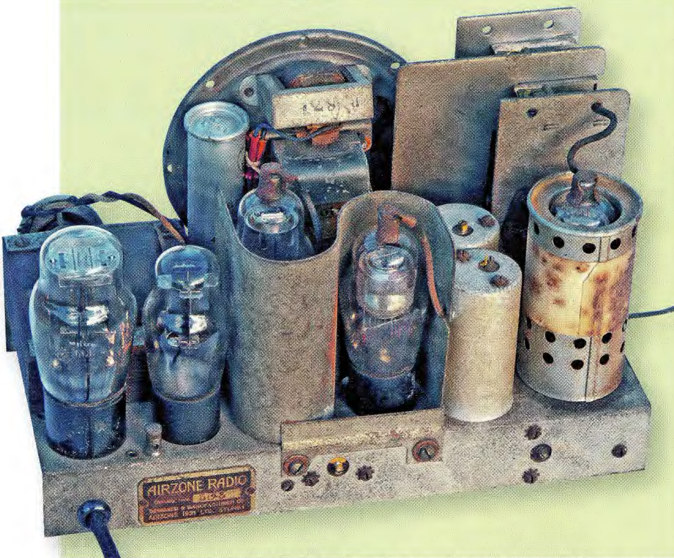
The top of the chassis is well laid out, with all parts easy to access for service. Note the unusual S-shaped metal shield between the IF amplifier (78) and detector (77) stages. A separate shield is also fitted to the mixer/oscillator stage.
