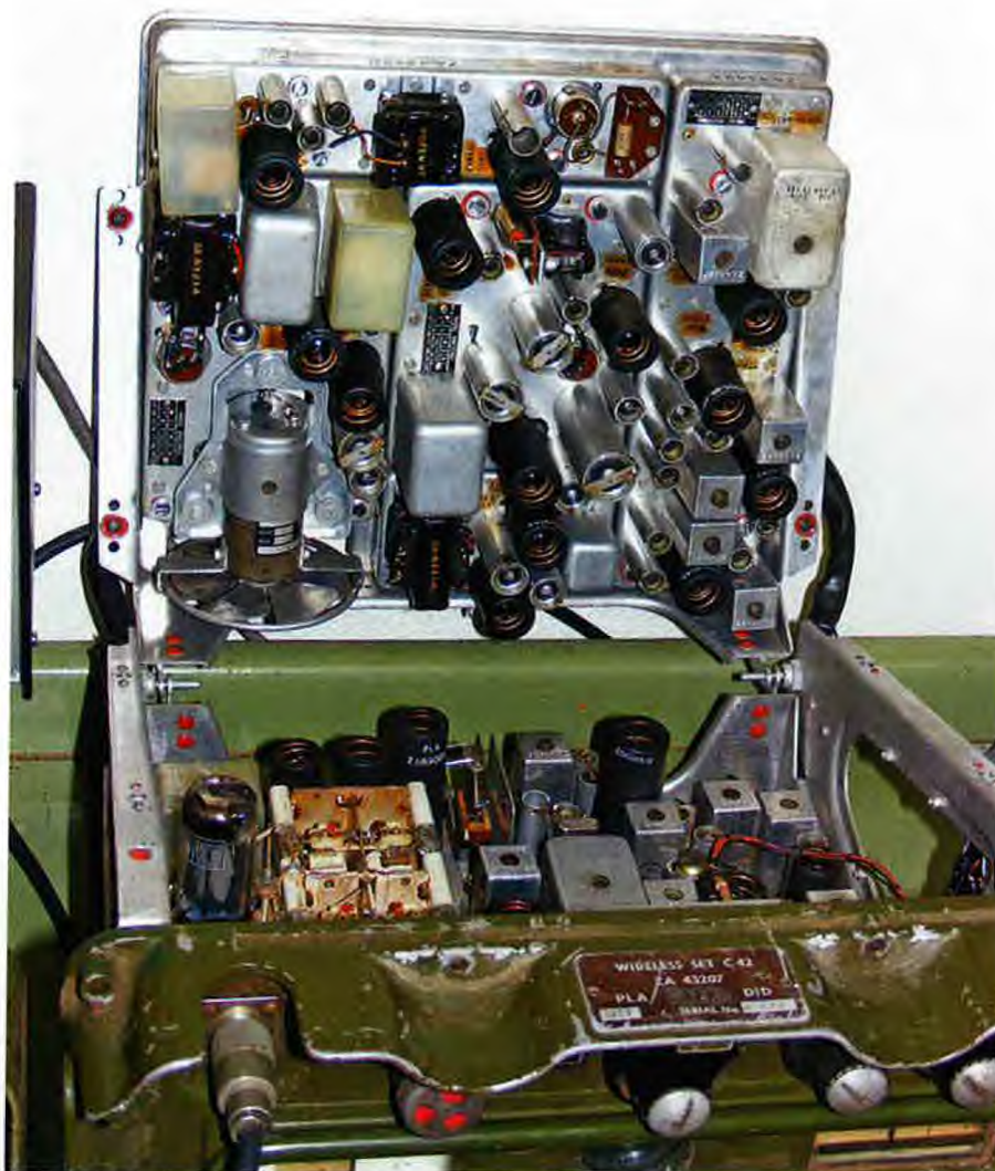
This Australian Army C42 military transceiver has 25 valves packed into a compact unit but is easy to open up for servicing.
