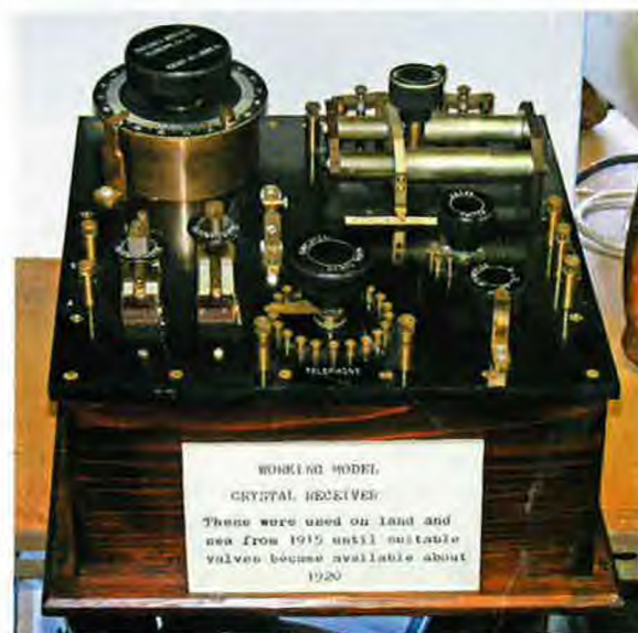
A replica 1915-era crystal receiver. These were widely used until valves became in the early 1920s.
