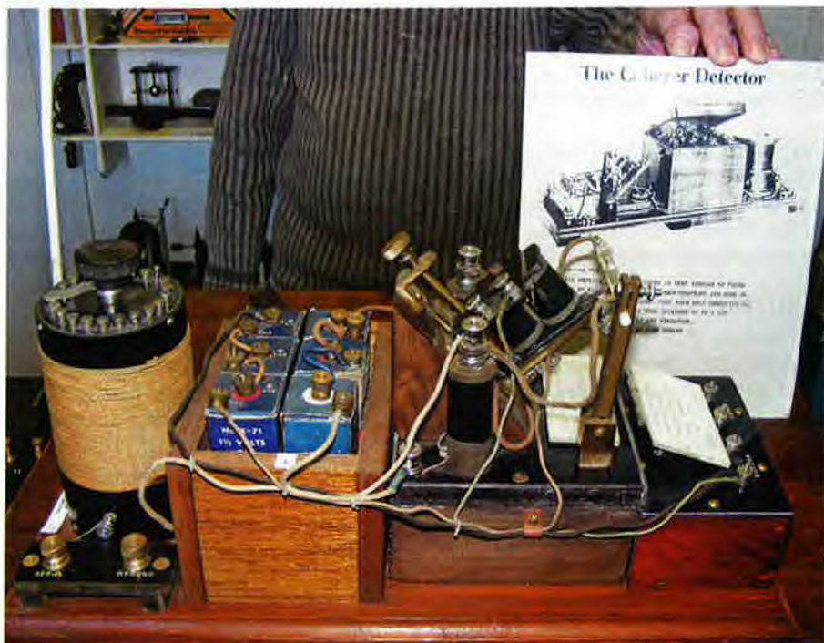
This working replica of 1902 coherer detector receiver is similar to those used by Marconi in the early days of radio.
