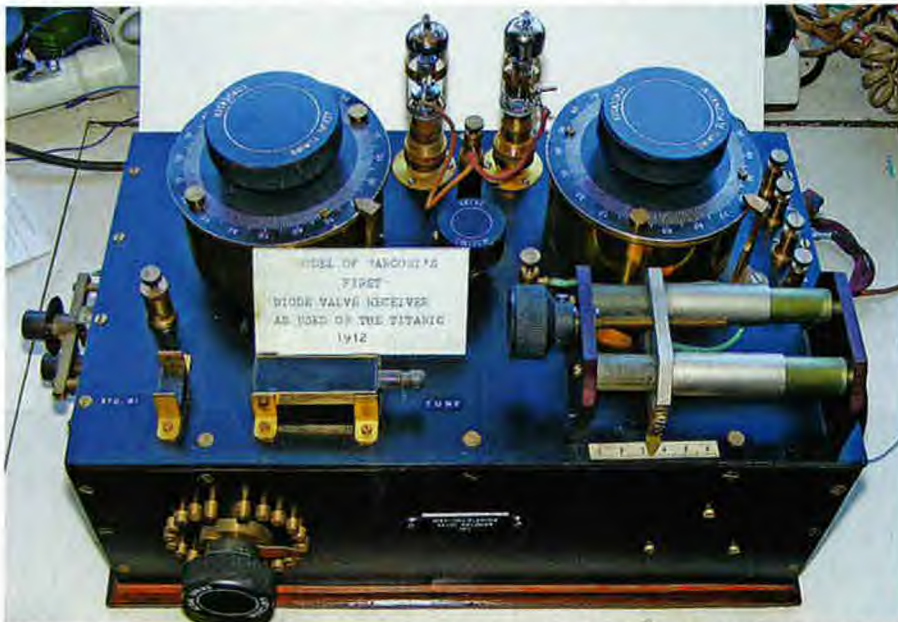
This working unit is a replica of Marconi's first diode valve receiver, as used on the steamship Titanic in 1912. Note the brass fittings used in this model.
