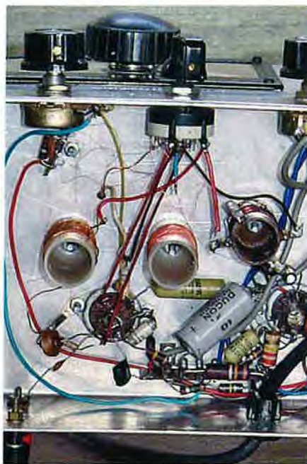
The coils are more widely spaced in David's set, leading to less interaction between them. The set performs quite well.
