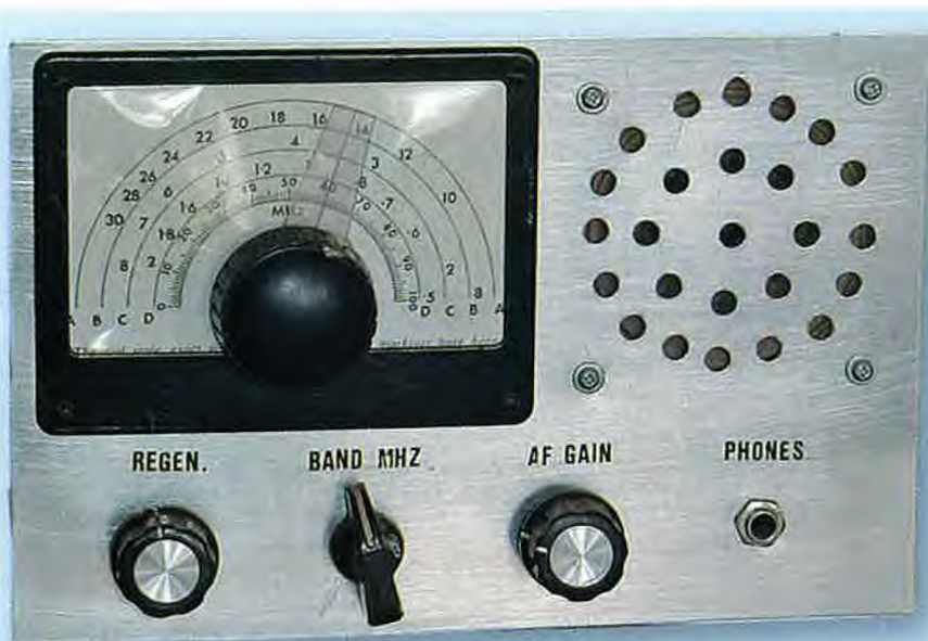
David's 1967 All-Wave-Two closely resembles the original "Electronics Australia" design. A cabinet will be necessary to protect the user from high voltages under the chassis
