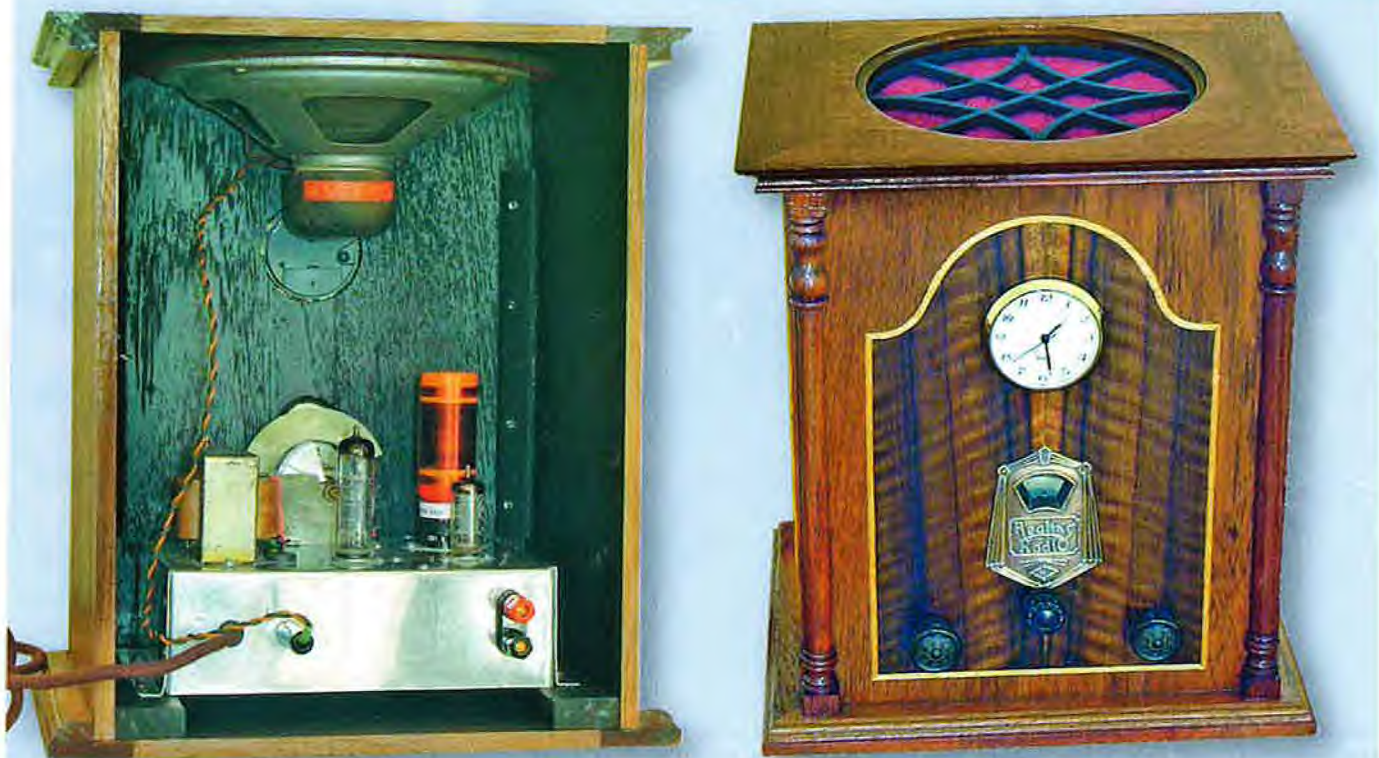
The high point of Dennis's set is its beautifully-crafted timber cabinet, complete with a clock and a keyhole dial escutcheon. The loudspeaker is mounted inside the cabinet facing upwards.
