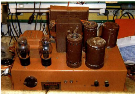
The chassis in good condition but some of the parts, including a 57 valve and an IF transformer, are missing due to its conversion to a simpler TRF circuit.
