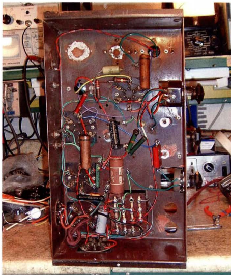
There is plenty of room under the chassis. Two holes at top left have been filled in by the previous owner, while the two large holes at bottom right originally accommodated the HT filter capacitors. Note the knot used to "anchor" the mains cord – a technique that's unsafe and completely unacceptable today.
