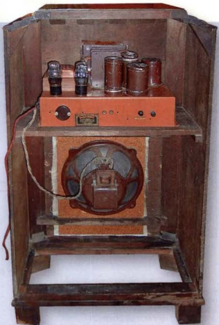
The chassis is bolted to a shelf inside the timber cabinet, while the electrodynamic loudspeaker is mounted on a heavy wooden baffle immediately below. The baffle isn't original though – it's made of chipboard, a material that didn't exist in the 1930s. The grille cloth has been changed as well.
