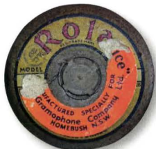
This speaker coil cover from another HMV radio illustrates how HMV rebadged the Rola speaker used in the model 209 and other sets.
