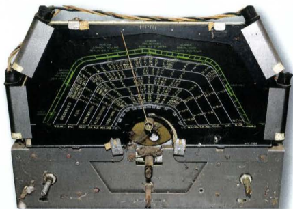
This view shows the front of the chassis and the dial prior to restoration. Despite its unusual shape, the large dial scale is easy to read.
