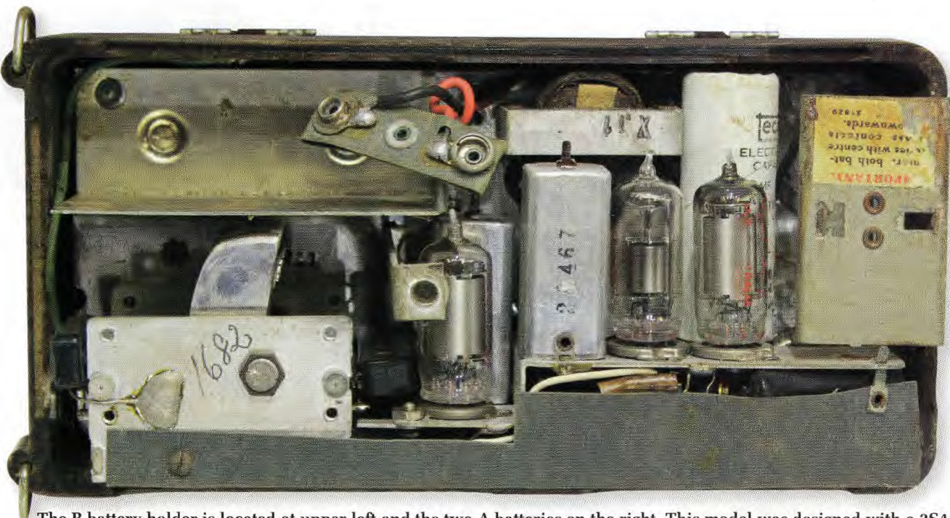
The B battery holder is located at upper left and the two A batteries on the right. This model was designed with a 3S4 pentode valve for the audio output stage, but due to its scarcity at the time, many models used a 1S4 instead.
