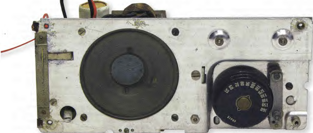
The front of the chassis is adorned by just the 3.5-inch speaker and tuning knob, with a tuning range of 540kHz-1600kHz. The volume control protrudes at lower left of the chassis.
