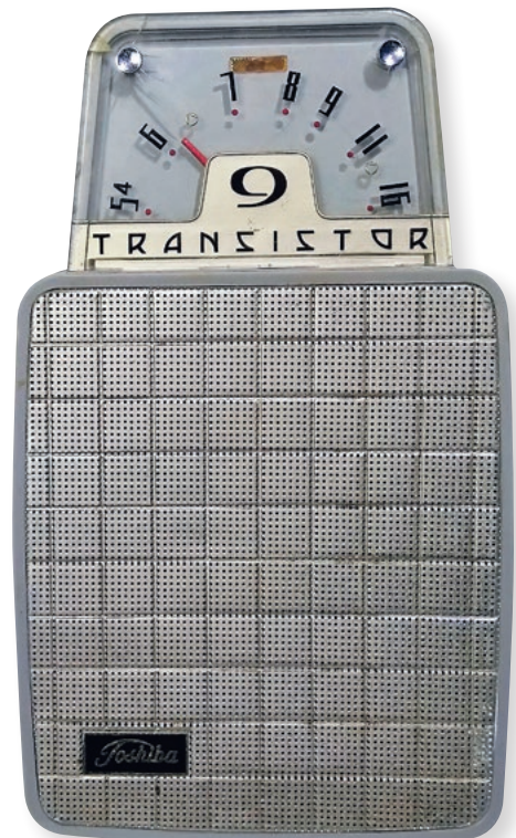
As the two screws on the front panel were easily over tightened, it was common for this panel to crack.
