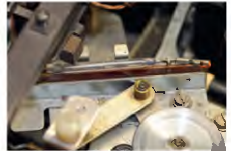
Fig.11: this reed relay is triggered by the tonearm when it approaches the record centre, indicating that playback is finished.
