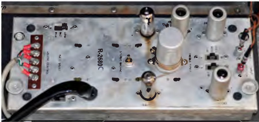
Fig.14: the preamp includes a magnetic cartridge amplifier and treble/bass presets for the installer to adjust.
