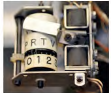
Fig.12: the annunciator wheels show the location of the currently playing record.
