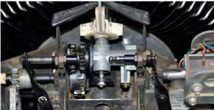
Fig.9: this set of gears is responsible for driving the transfer arm and positioning the tonearm over the starting track of the record on the turntable.
