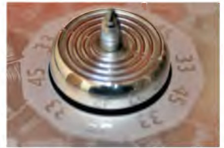
Fig.10: this mechanism detects whether the record is a 33RPM or 45RPM type, and adjusts the turntable speed accordingly.
