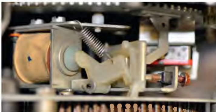
Fig.7: these microswitches are responsible for stopping magazine rotation when the selected record is reached, by detecting the pin sticking out.
