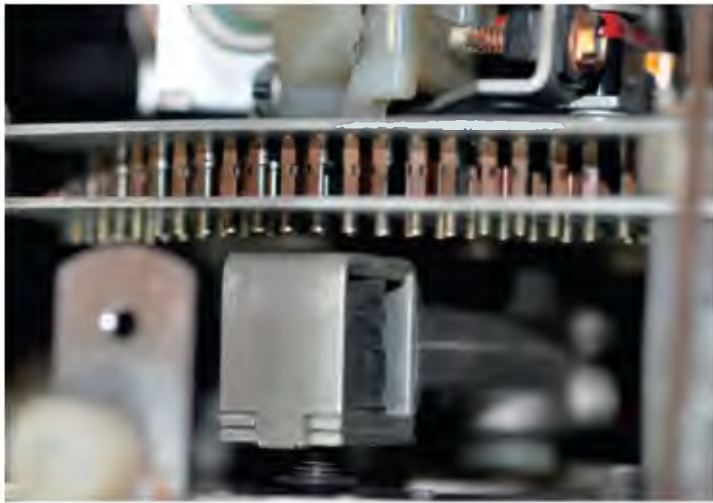
Fig.5: one of the 'pin pusher' solenoids used to cue a record to be played.
