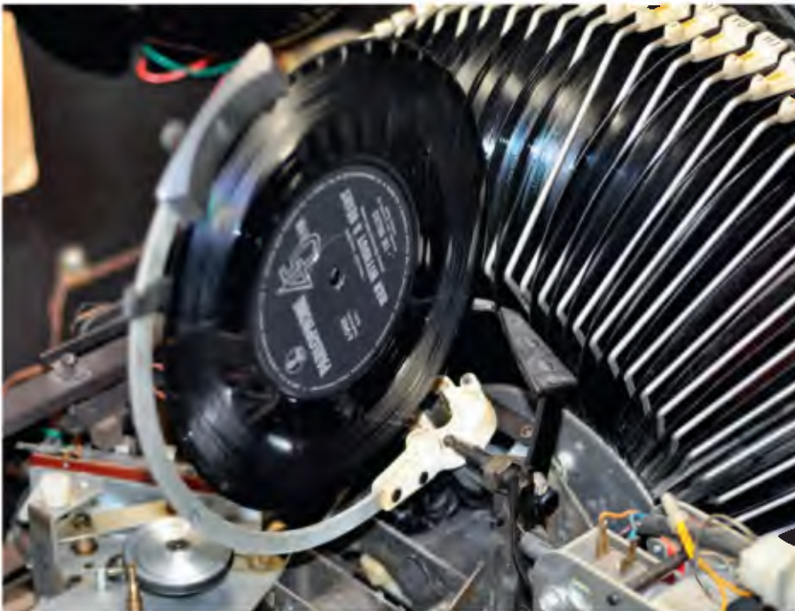
Fig.8: a record being lifted out of the magazine by the transfer arm, ready to drop onto the turntable.
