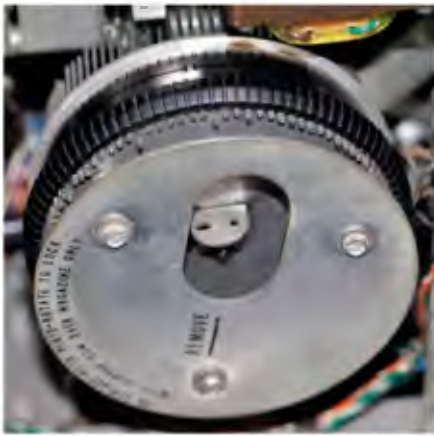
Fig.17: this 'popularity meter' pushes in the pin corresponding to a given record a little bit each time it is played. Thus, the pins sticking out further correspond to records that have been played more times.
