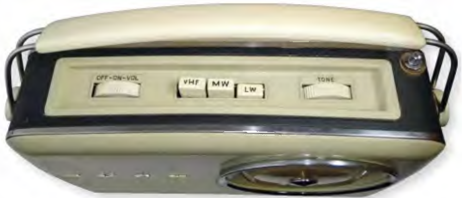
The top view of the case shows the volume control (which doubles as the power switch), band change selector, tone control, and the telescopic aerial.
