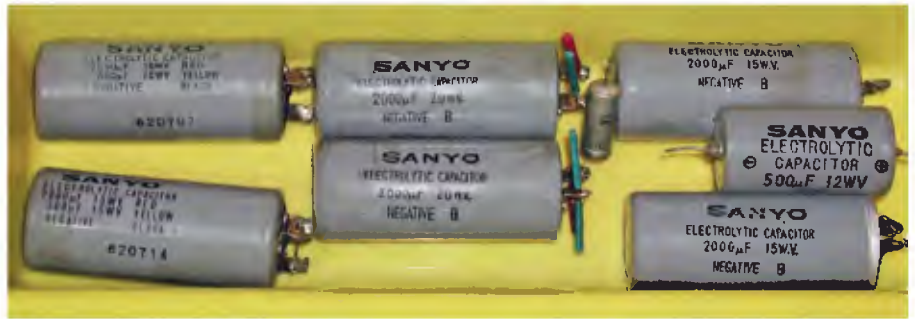
The original Sanyo capacitors (shown approximately half size) used for power supply filtering etc, had failed when the set was powered on. The 500 \mu F capacitor at right is the coupling capacitor for the vertical yoke's coils. The rest of the 2000 \mu F capacitors were replaced with 4700 \mu F Nichicon types shown below (actual size), as they were the closest in terms of appearance and size.
