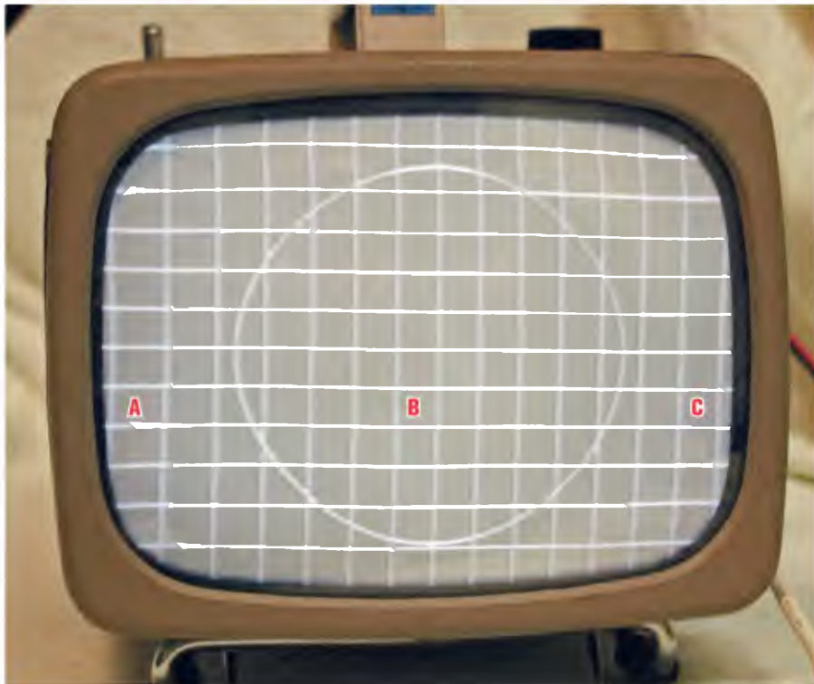
The horizontal linearity of the Sanyo 8-P2 is not as good as the adjacent Sony TV (for example region "A") despite it having an S-correction capacitor.
