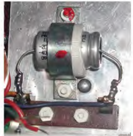
The yoke coupling capacitor was replaced with this Rifa 1000 \mu F automotive capacitor.
