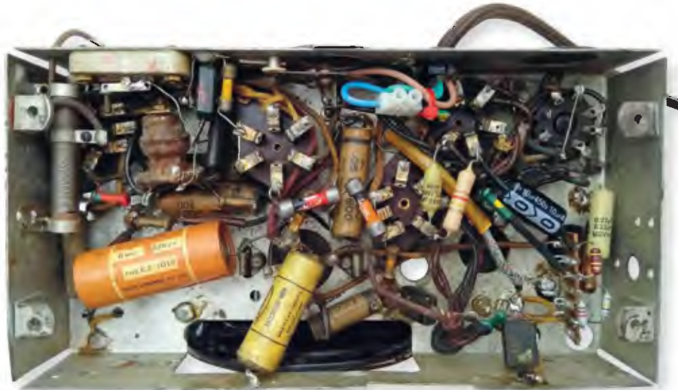
The vacant space in my set and the chassis hole to the right would have been occupied by the internal/external speaker switch on earlier releases. No original electrolytic capacitors remain in my set.
