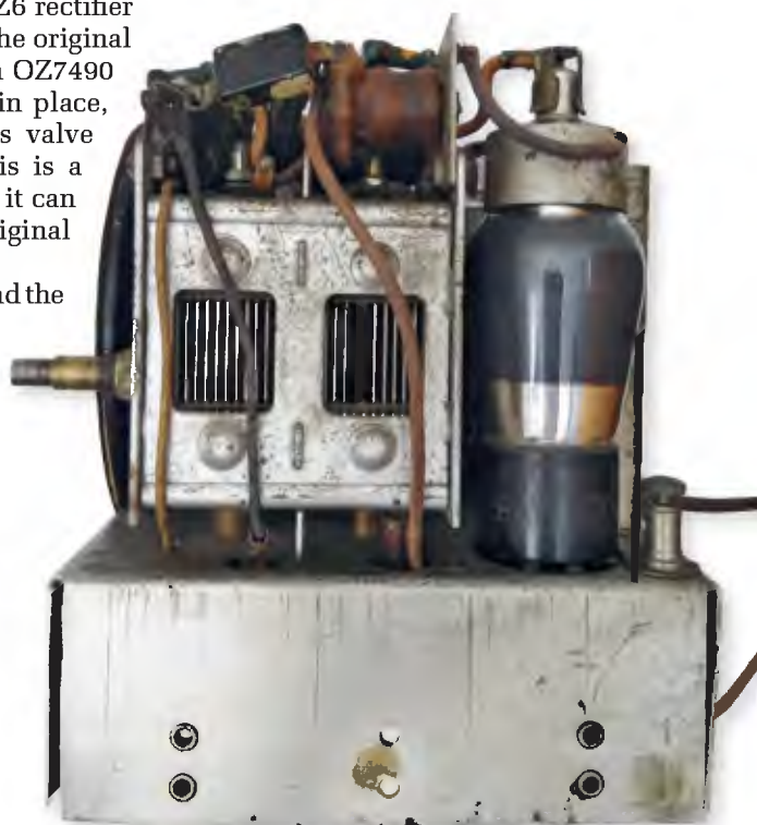
The side view of the Astor Mickey OZ clearly shows the filter circuitry for the antenna.
