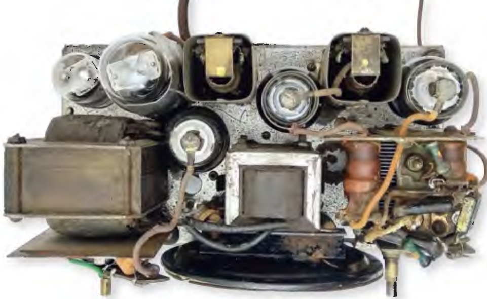
The top view of the chassis gives a better look at the 'messy' arrangement near the tuning gang which is for the antenna circuitry.
