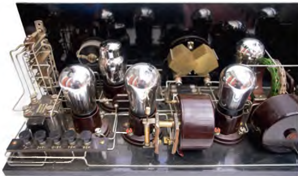
A close-up of the left side of the radio chassis, from left-to-right are the Thordarson coupling transformers, grid leakage detector, 4th & 3rd IF transformers, plus the oscillator coils at the back (green/white wire).
