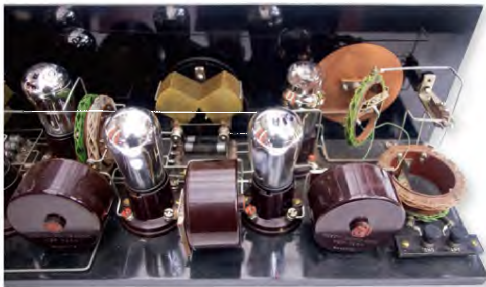
A close-up of the right side of the radio chassis, again the 3rd IF transformer is in view, along with the 2nd and then 1st (A-type) followed by the aerial coil. Behind that is the "sensitizer" regeneration control.
