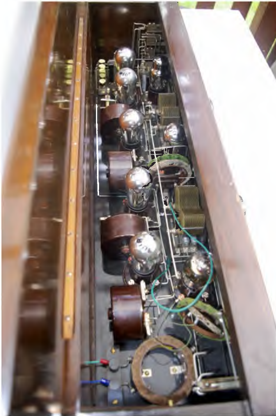
The interior of the L-2 is nicely designed, with most components mounted on the timber “breadboard” and connected via point-to-point wiring. Considering this radio was originally designed in 1922, the layout is impressive.
