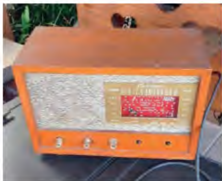
Figs.1 & 2: the Calstan (also known as Slade) 559M2 radio was initially provided in 'worn' state, with some knobs missing and the dial a bit scuffed.
