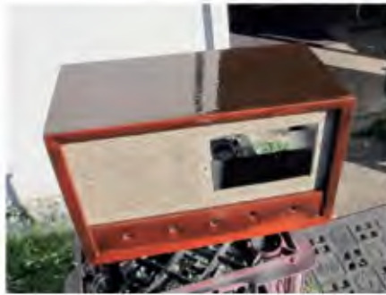
Fig.9: a fabric cleaner was used on the front panel cloth, and a gloss coat to the timber cabinet.
