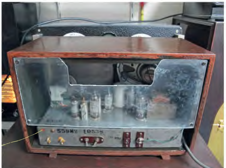
Fig.11: the chassis was then remounted inside the cabinet with the MSP speaker, measuring 9 x 6-inches and rated at 15Ω. After mounting the chassis, the rear of the cabinet was sealed with a piece of clear Perspex as a safety measure (see the photograph below).
