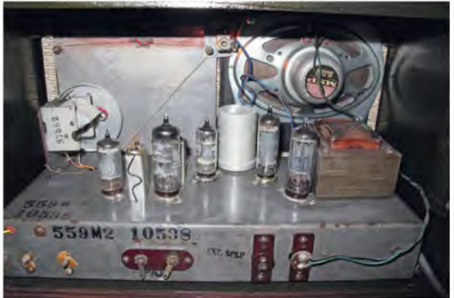
Fig.11: the chassis was then remounted inside the cabinet with the MSP speaker, measuring 9 x 6-inches and rated at 15Ω. After mounting the chassis, the rear of the cabinet was sealed with a piece of clear Perspex as a safety measure (see the photograph below).
