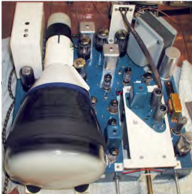
The top of the chassis post-restoration. The only components mounted on this side are the valves, CRT and transformers, lending it a tidy appearance.
