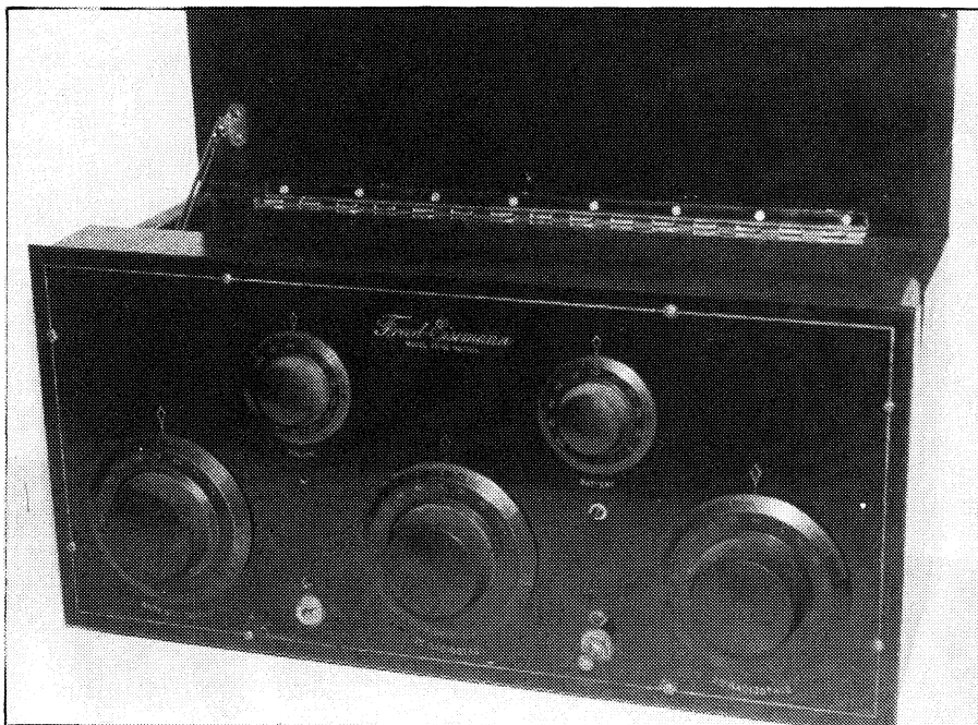
The 1925 Freed Eisemann was a typical 5-valve TRF, with 3 tuning controls and 2 filament rheostats for controlling gain. The hinged lid was almost universal at this time.
