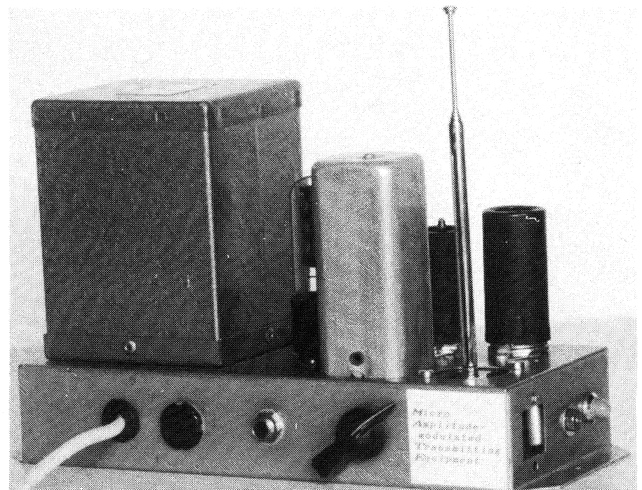
The author's prototype for the 'MATE' mini-transmitter, built on a disused power supply chassis.
