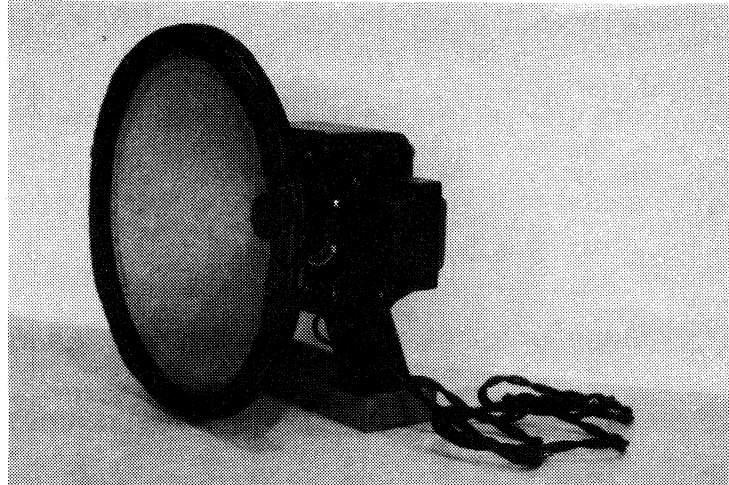
For its day, the 12" loudspeaker was progressive, with the centring 'spider' behind the zinc sputtered cone. Note the output transformer on the side.
