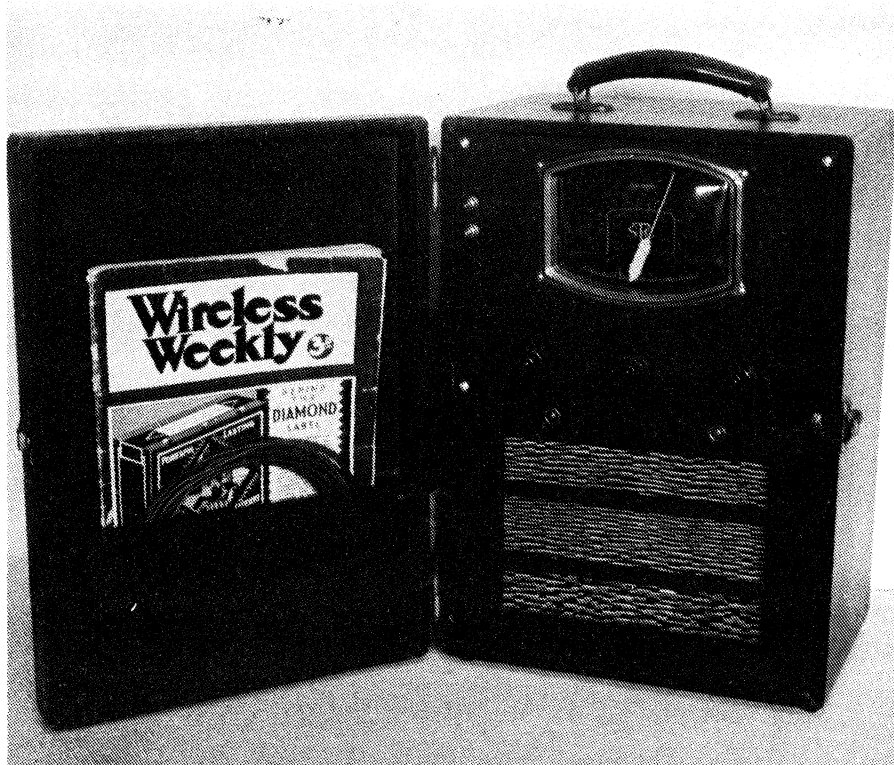
Portability, 1939 style! The batteries were housed behind the speaker grille. Instead of a loop aerial, a coil of wire was unwound and suspended from a suitable tree or building.
