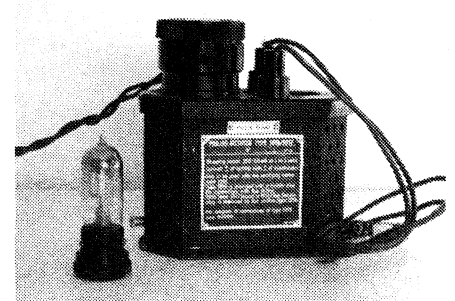
Fig.2: The companion Philips 1017 trickle charger for 'A' batteries, with its tiny mercury vapour rectifier.
