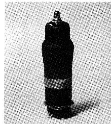
Fig.1C: After re-gluing the base and coating the wire with epoxy resin, cover the repair with a strip of tape or paper.
