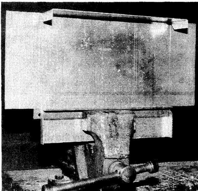
**Above: Folding the chassis with two lengths of angle iron in the vice — the front piece being a few millimetres shorter than the side being bent. At right are the dimensions for the original 1940 chassis, which may need to be varied to suit your components.**
