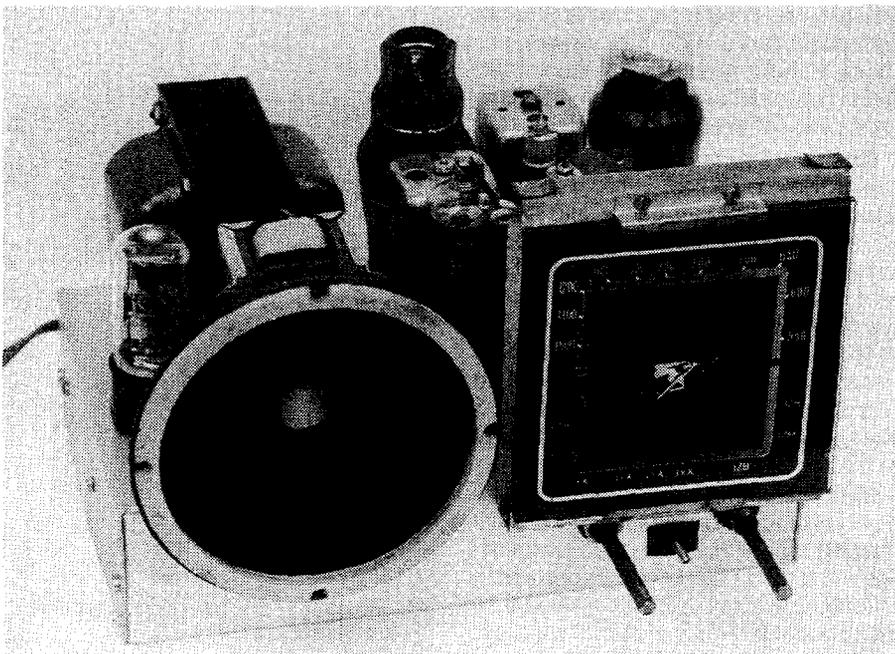
*The completed chassis. A similar layout was used for all versions, with exact dimensions and orientation dependent on the size of the main components. 6G8-G and 6B8-G IF valves require shielding — this chassis uses a 'goat' type shield (centre rear), which John Moyle also used in the original.*
