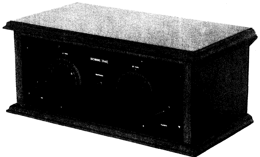
Home built Browning-Drake receivers were to be found in all manner of cabinets. This table top chest with lift-up lid was a popular pattern.
