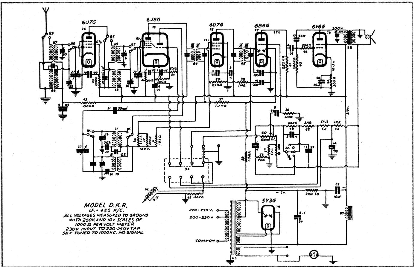
It is clear from this 1940's radiogram circuit that Astor produced well engineered, conservative designs. An advanced feature, as mentioned by Douglas Bolton in his comments about enhanced reproduction, is the elaborate negative feedback network, connected to the tapped volume control, and providing a degree of bass and treble accentuation. Resistor 52 (5k) is shorted out in the gramophone position to produce still more bass boost for pickup equalisation.
