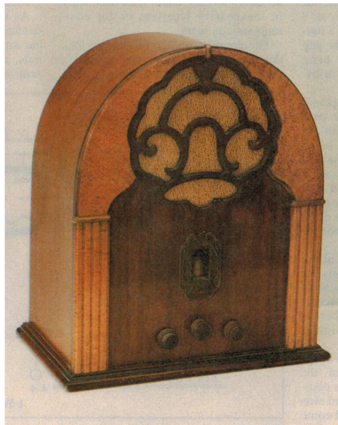
Curved top 'Cathedral' receivers from the period 1931 - 33 are very popular with collectors. Many, like this 1931 'Zenette' LH, used a biased detector.
