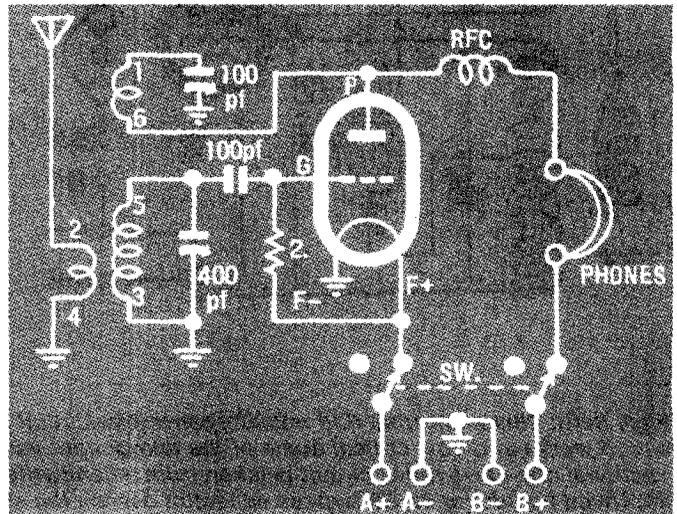
**Fig.4: The circuit for a one-valver intended as a training exercise for a beginner, described in 'Radio and Hobbies' for September 1954.**
