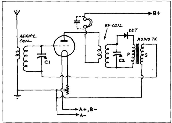
**Fig.1 (left):** This somewhat odd reflex/regenerative circuit appeared in 'Wireless Weekly' for October 21st, 1927. How the circuit works and how critical some of the component values were is explained in the text. **Fig.2 (right):** This more conventional one-valve reflex circuit is taken from a handwritten notebook of about 1927. Its performance could probably be improved by adding an RF bypass capacitor across the audio transformer secondary winding.
