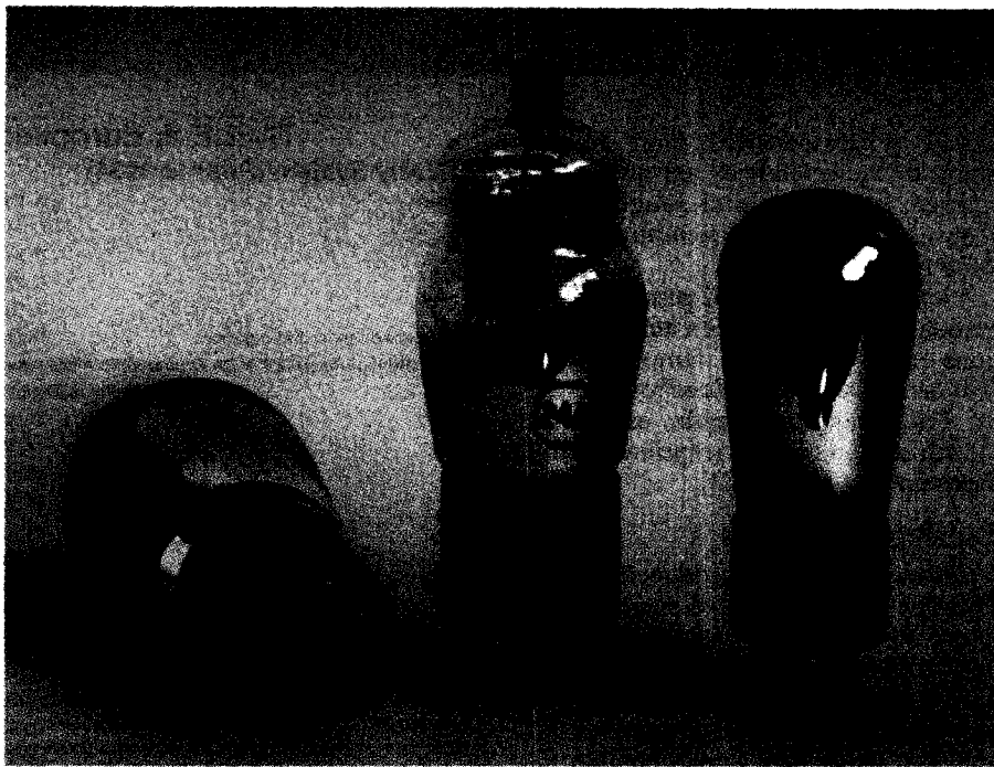
Three relatively early American valves. On the right is a type 30 battery triode with a 'UX' type four-pin base, while in the centre is a type 24A indirectly heated 2.5V RF tetrode and at left a type 47 directly heated 2.5V output pentode — both using the 'G' envelope with a five-pin base.
