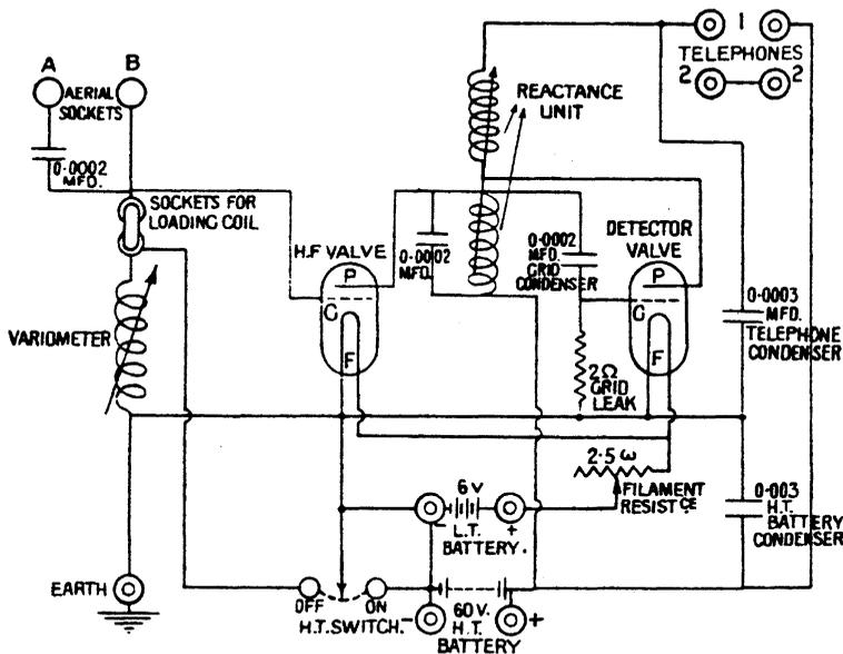
Fig.1: The circuit of the Gec-o-Phone model BC 2001.
