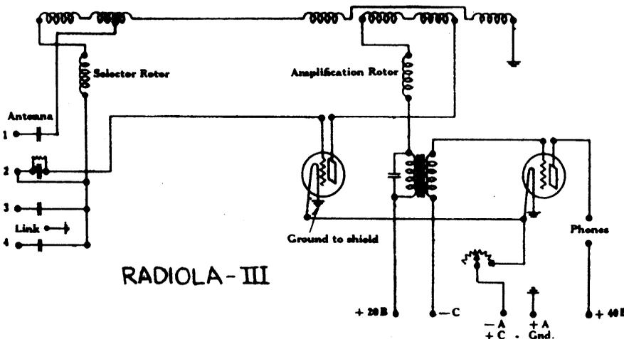
Fig.3: The circuit of the Radiola III two-valver.
