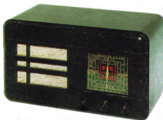
Fig.1: The Healing 408A four-valve mantel radio of 1938, which uses a vibrator power supply.
