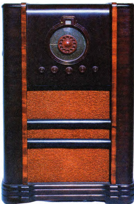
Fig.2: The Healing 668A dual wave six valve console set, also of 1938 and vibrator powered. It's a very good performer.
