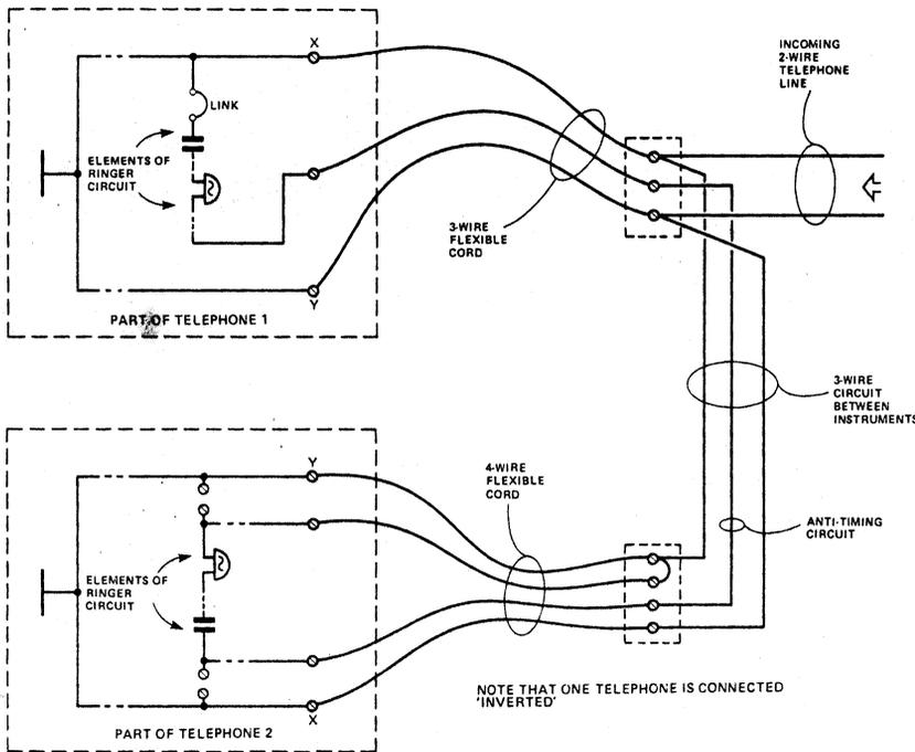
**Figure 6: Typical wiring plan for telephone extensions. The 3rd wire (sometimes called 'the shunt wire') forms part of the sometimes quaintly termed 'anti-tinkle' circuit.**
