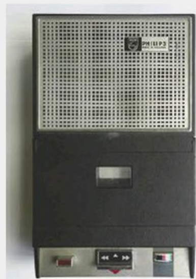
Above: The shoebox-style Philips EL3300 was the very first Compact Cassette recorder (Image credit: Erkaha, CC BY-SA 4.0).
