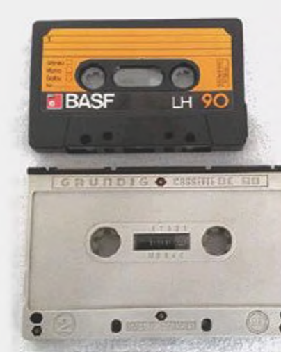
Below: Grundig's DC-International cassette was a brief competitor during the mid-1960s (Image credit: Ulrich Miemietz, CC BY-SA 3.0).
