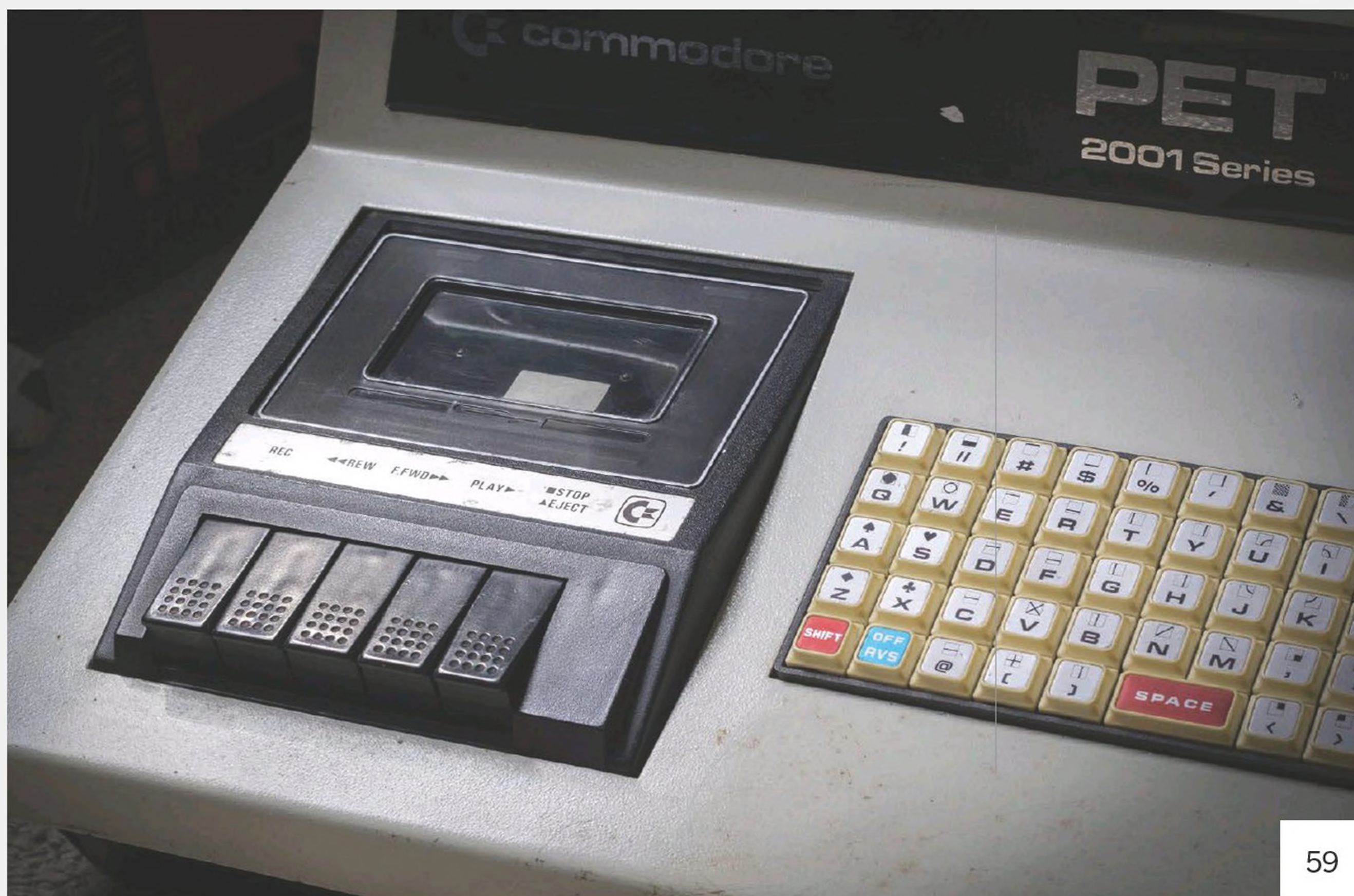
Below: Compact cassettes featured in 1970s' home computers, including the Commodore PET (Image credit: Parrot of Doom, CC BY-SA 4.0).
