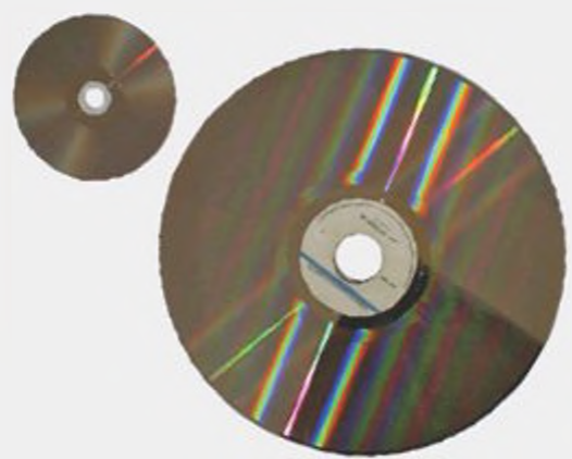
Above: LaserDisc stored analog video on optical discs 30cm in diameter (Image credit: Kevin586, CC BY-SA 3.0).
