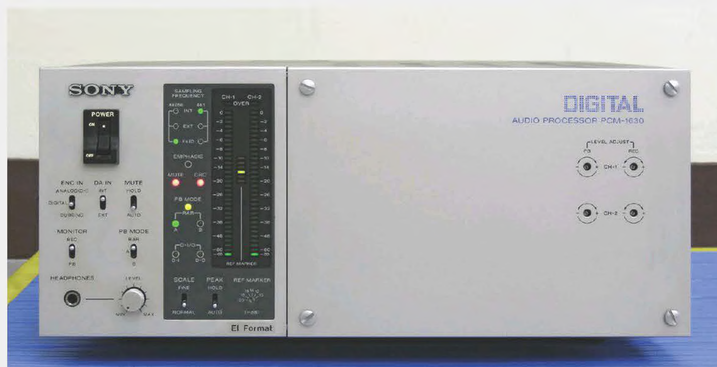
Below: The Sony PCM-1630 PCM adapter turned any VHS recorder into a digital audio recorder (Image credit: Akakage1962, CC-BY-SA 3.0).
