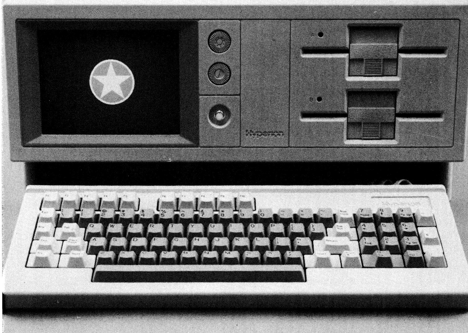
The Hyperion computer features a built-in video display, dual disk drives and a low-profile detached keyboard.
