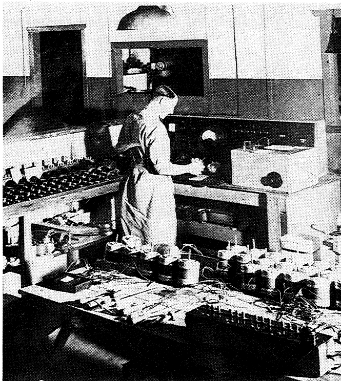
Left: Quality control at Byer Industries. Factory foreman Jack Richardson checks a batch of motors and other components being readied for final assembly. Right: In sharp contrast to the 'Junior' portable recorder, a batch of multi-speed professional turntables are seen undergoing a mandatory two-hour test run for heat rise above ambient.
