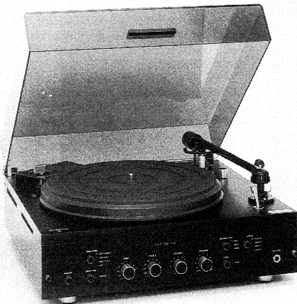
Fig.6: A solid state Saraband amplifier/record player. Produced around 1989, and intended for record collectors, it is fitted with a precision multi-speed turntable capable of playing 33/45/78/80rpm discs. It is provided with Equidyne arm, raise/lower lever and provision for interchangeable heads.
