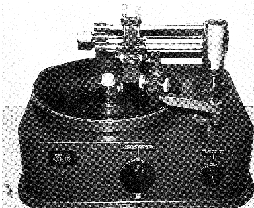
Fig.4: One of Vic Harris' early recording lathes, in Peter Stinson's collection of MBH memorabilia. Note the on-board microscope and the identity plate, which identifies it as Model G2, by Victor Harris of Knocklayde Street, Ashfield.
