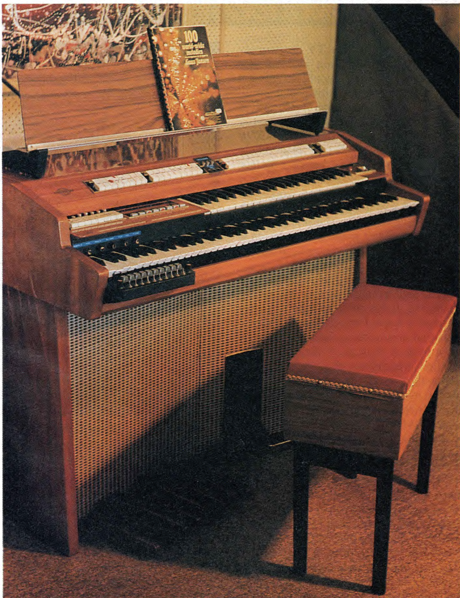
Arthur Spring's experimental organ, tidy but never 'finished'. Because his wife is a trained pianist, it is fitted with a full piano lower keyboard with access to electronic piano as well as organ voices.
