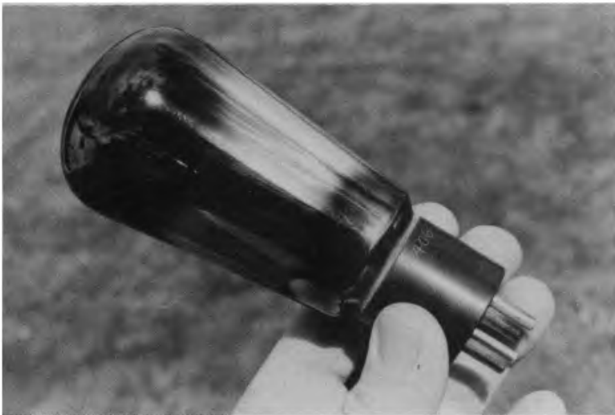
Big was beautiful back in the good old days. Shown is an E406, an early AC output valve. The type number has been scratched into the base for identification.
