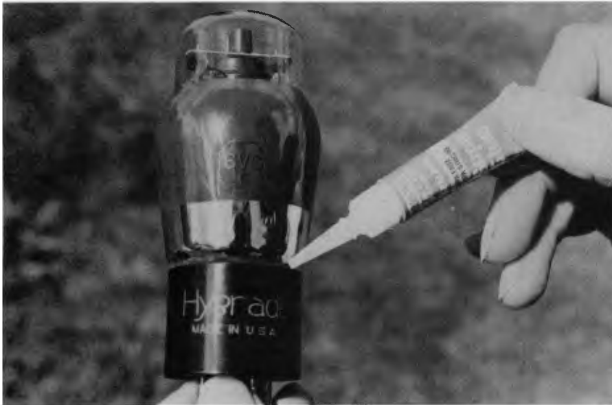
Loose valve bases can easily be repaired with a few drops of "Super Glue". In some cases, it may also be necessary to resolder the pins.
