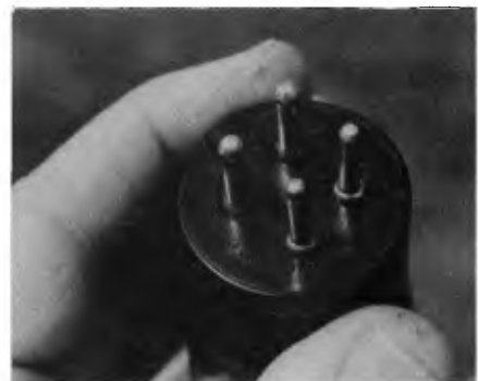
Resoldering the base pin connections will often bring a faulty valve back into service. Remove the old solder and clean the wires and base pins before resoldering.
