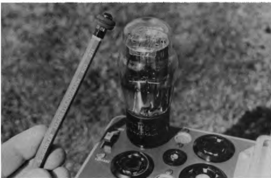
A valve should be gently tapped during testing to show up any intermittent faults. A rubber grommet fitted to the end of a pencil makes a suitable valve "donger".
