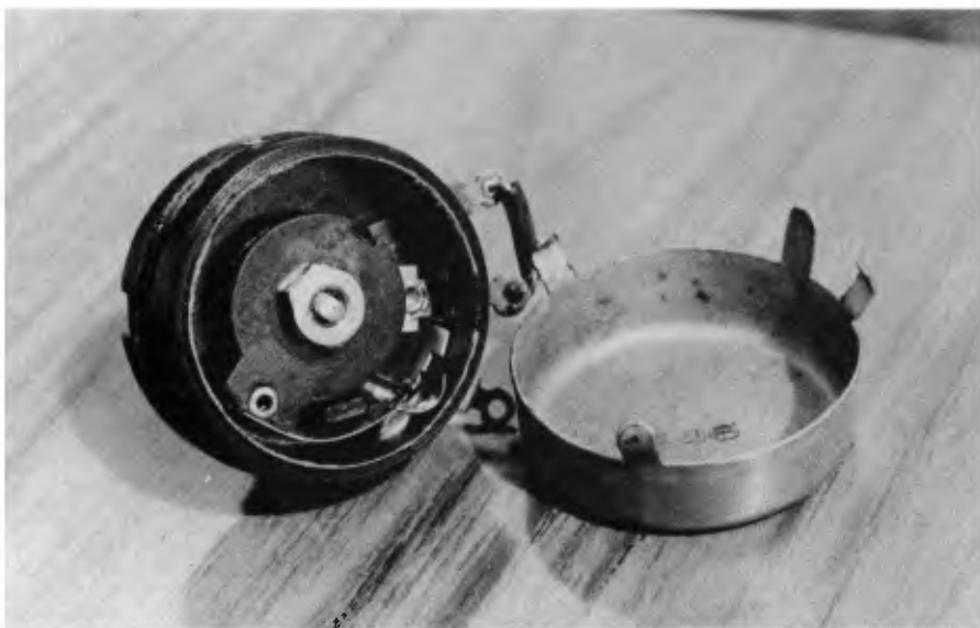
A noisy pot can often be cured by spraying WD40 or similar cleaning fluid onto the carbon track. For early pots, the dust cover must first be removed for the treatment to be effective.
