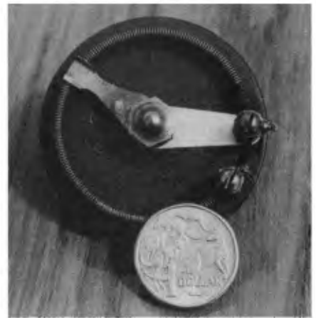
Rheostats (or variable resistors) were used in early battery radios to regulate the filament voltage. These units are typically quite robust and seldom require replacement.
