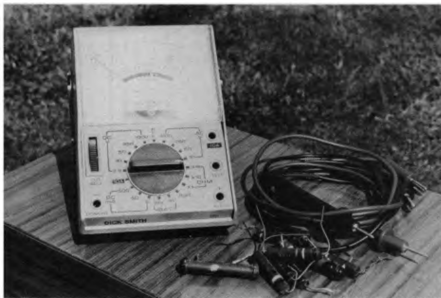
A good multimeter is essential for checking resistor values. When restoring a vintage radio, it is a good idea to check the value of every resistor in the circuit as a matter of course.
