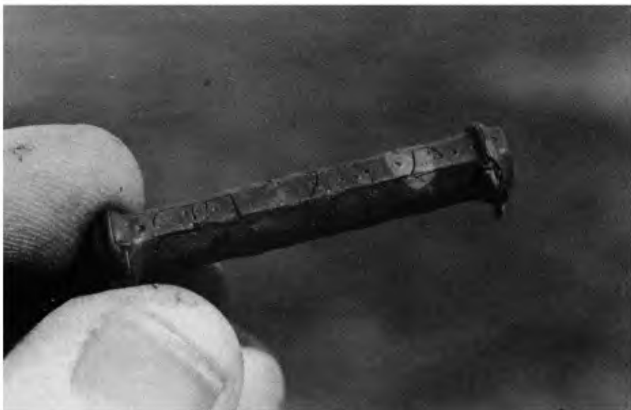
A burnt out resistor is a fairly common problem in valve radios and generally occurs when some other component (eg, a capacitor) breaks down.
