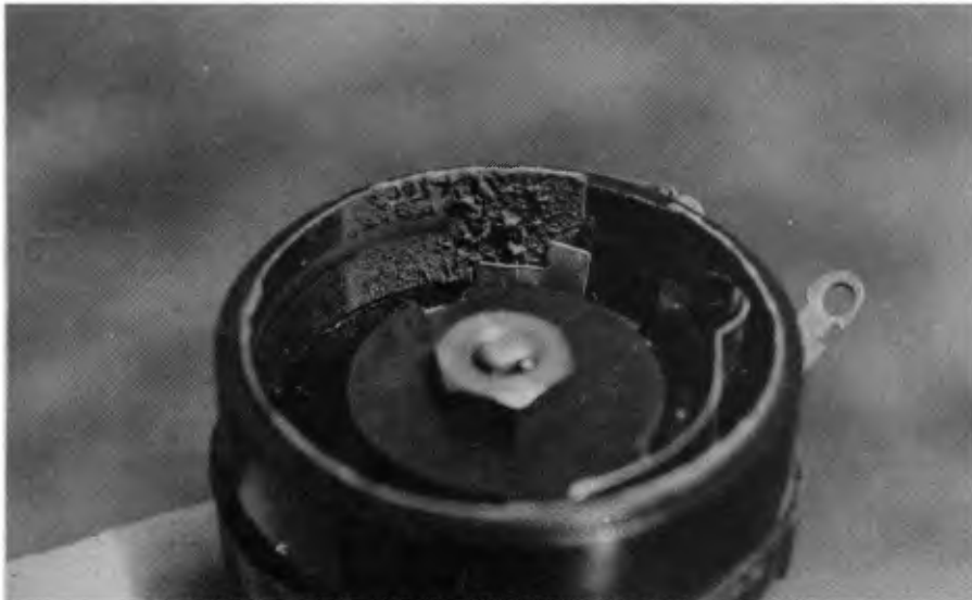
It's not hard to see why this carbon pot was giving trouble. Excessive power dissipation, probably due to an external component failure, has "cooked" the carbon track. Pots in this condition must be replaced with an equivalent type.
