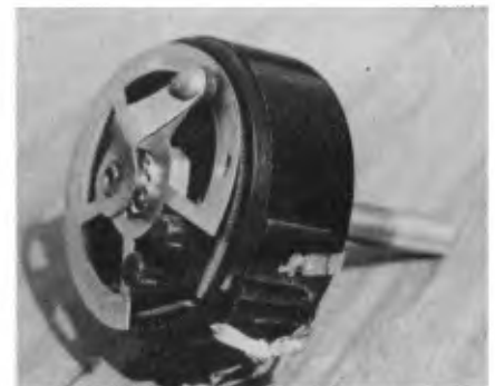
A typical wirewound potentiometer from the 1930s. These can give trouble due to dust and dirt in the works. A careful clean followed by a spray with WD40 will usually restore the pot to as-new condition. The wiper arm requires periodic lubrication.
