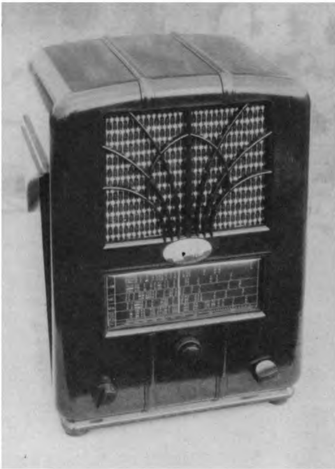
An early post-war HMV 5-valve receiver. Once again, many hours of work have restored the Bakelite cabinet to as-new condition. These old sets were capable of good performance.
