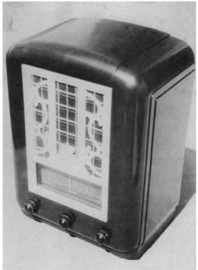
This 5-valve Airzone is a classic mantle radio from the late 1930s. This particular set is housed in a Bakelite cabinet and features a rather ornate loudspeaker grille insert.
