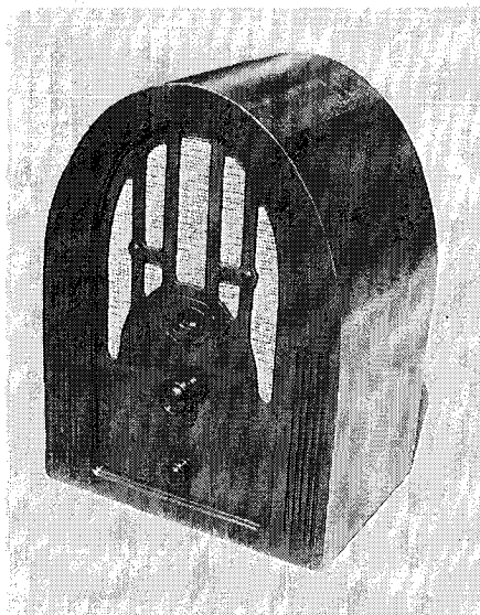
Many superhets from the early 1930s, such as this 4-valve Airzone, also lacked automatic gain control. Next month, we will describe an AGC conversion for this particular receiver.
