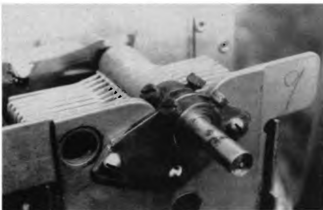
The tuning capacitor is a plain bearing type with two collars & set screws to control end float. Plain bearing tuners often require cleaning & lubrication if they are to work smoothly.
