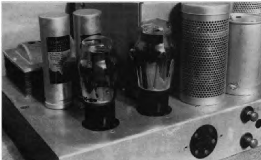
This view shows the 80 rectifier valve (left) & the 47 output valve. The chassis cleaned up quite well for a 60-year old receiver. The two terminals at bottom right are for a gramophone pick-up.
