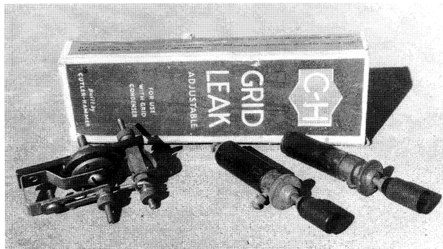
These variable grid leak resistors are real relics from the past. The one on the left has a carbon track & wiper arm, while the others are, presumably, carbon granule compression types.
