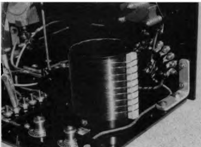
The parts visible in this photo include the tapped RF coil, the rear of the stud switch & the trimming capacitor. The alligator clip at the left is used for selecting the detector coil taps & once set rarely needs shifting.
