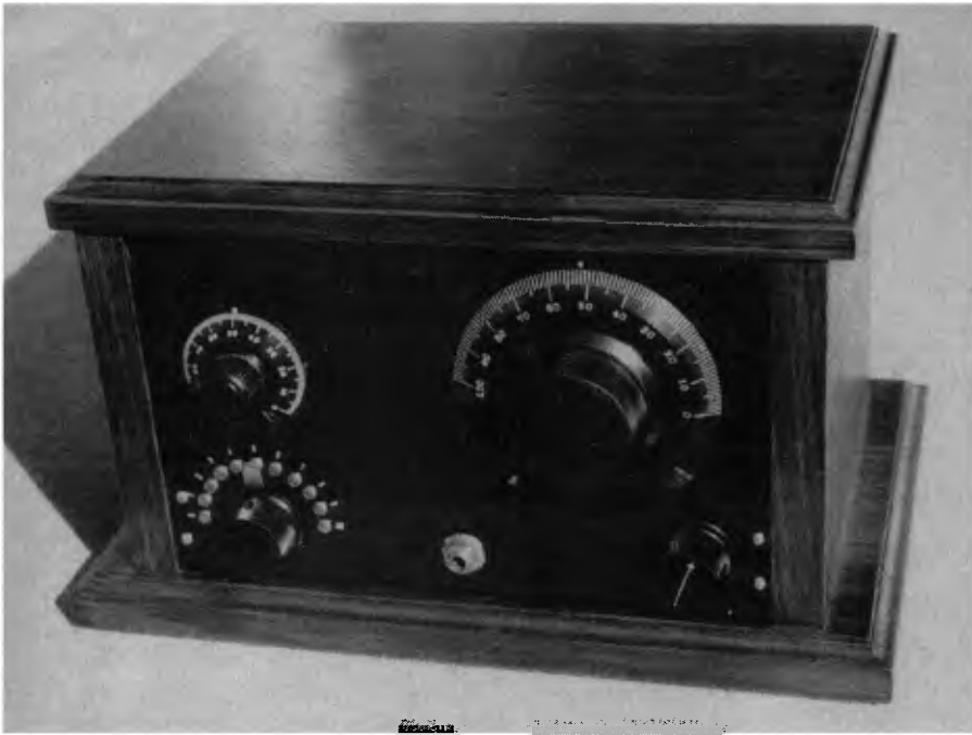
The finished receiver successfully captures the vintage look of the 1920s. The crystal detector was mounted high on the back of the front panel where it is out of harm's way.
