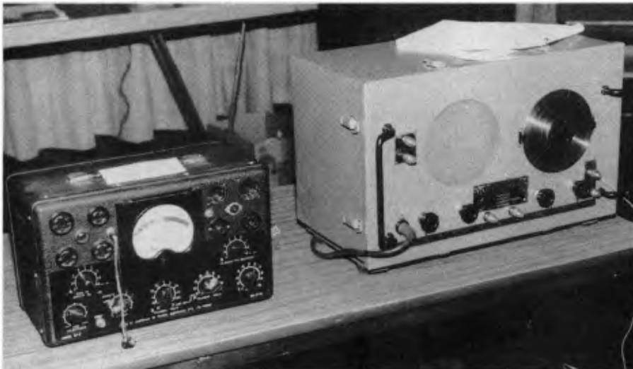
This table carried an old Palec valve tester & what appears to be an early Stromberg-Carlson communications receiver.
